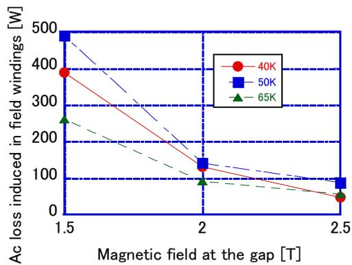
Fig. 7. The ac loss induced in field windings
