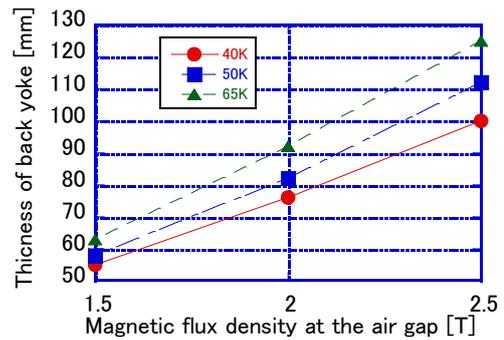
Fig. 5. Required thickness of back iron yoke.
