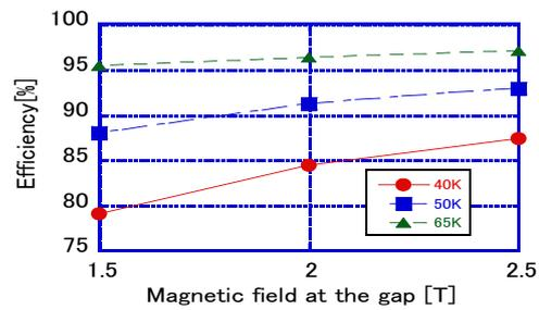
Fig.9 . Calculated the efficiency of fully superconducting motors.
