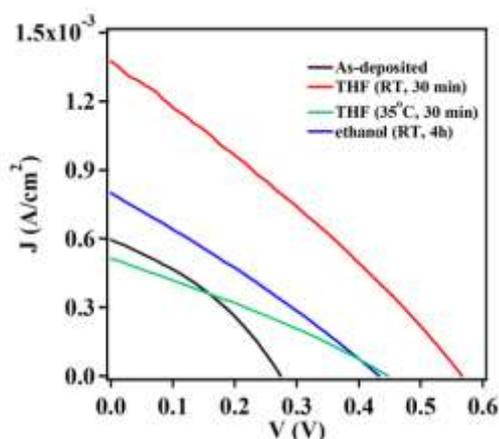
**Figure 4** J–V characteristics of ZnO/TiOPc/DH-a6T hybrid solar cells at various annealed solvents of TiOPc thin films under AM1.5G simulated illumination ( $100 \text{ mW/cm}^2$ ).
