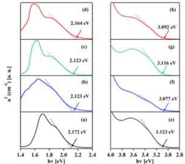
**Figure 3** The photon energy dependence of  $\alpha^2$  for TiOPc thin films before (a, e) and after solvent vapor annealed with (b, f) THF (RT, 30 min), (c, g) THF (35 °C, 30 min) and (d, h) ethanol (RT, 4 h), respectively.
