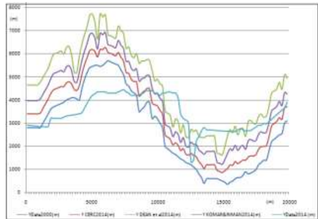
Fig. 3: The result of running model of shoreline change for three difference formulations of; Dean et al. [2], Komar-Inman [6], and CERC [3] and [8]
