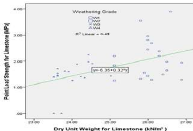
Figure 19: Relationship between point load strength and dry unit weight with weathering states.
