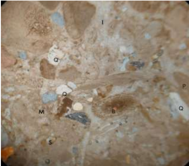
B – Bioclast, Q – Quartz, P – Pellet, M – Micrite, I – Intraclasts, S - Sparite
