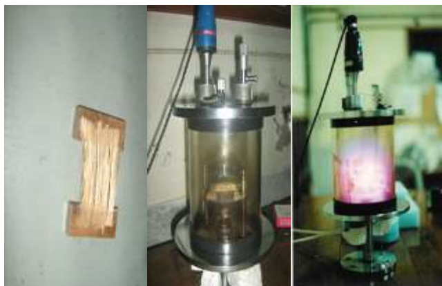
Fig. 1 Schematic diagram of jute fibre and position of it in the glow discharge reactor
