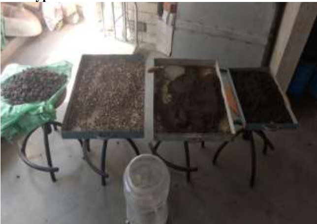
Fig. 16: Materials used in slow sand filter
