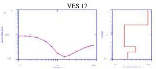
Fig 18. Curve matching with model of VES 17
