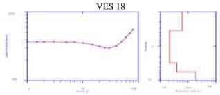
Fig 19. Curve matching with model of VES 18
