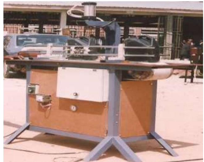
Fig 15: Photograph of sealing machine
