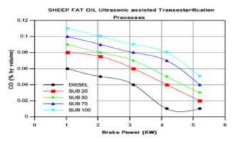
Figure 5. CO emission against Brake power
