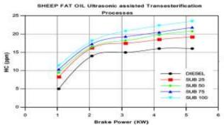
Figure 6. Hydrocarbon emission against brake power
