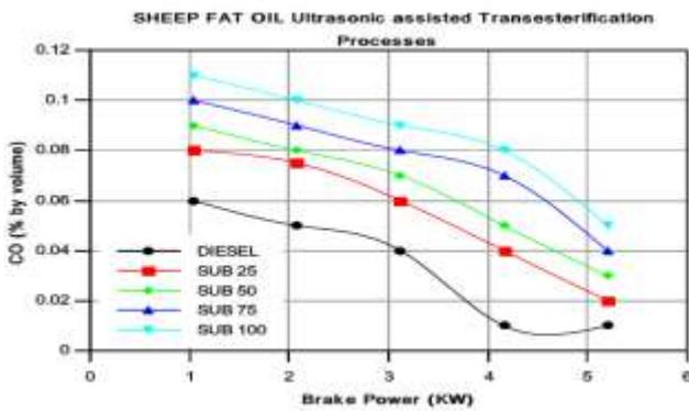
Figure 5. CO emission against Brake power
