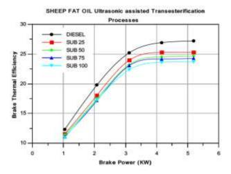
Figure 4. Brake thermal efficiency against brake power
