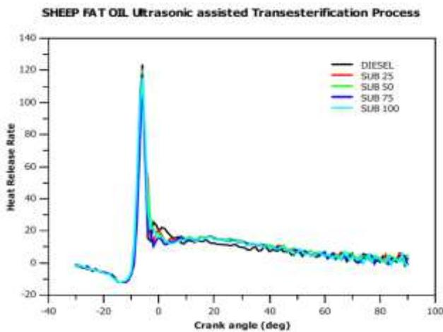
Figure 10. Heat release rate against crank angle
