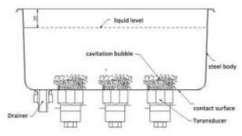
Figure 2 Schematic diagram of ultrasonicator assisted Transesterification process
