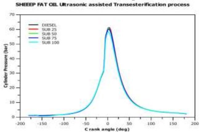
Figure 9. In-cylinder pressure against crank angle
