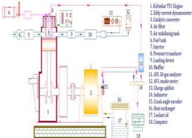
Figure 3. Schematic diagram of the experimental setup
