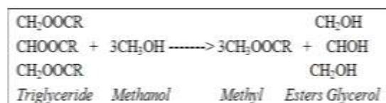
Figure 1 Transesterification process of converting Sheep fat oil to biodiesel
