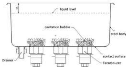
Figure 2 Schematic diagram of ultrasonicator assisted Transesterification process
