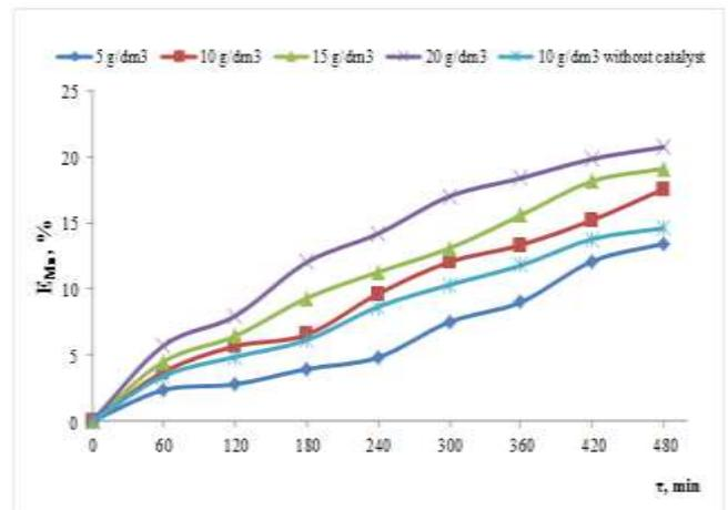
Figure 4- Degree of manganese extraction during leaching of mill tailings depending on the concentration of sulfuric acid in the presence of a paramagnetic catalyst
