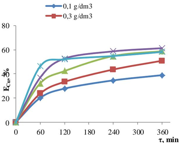
Figure 6 - Extraction degree of copper from mill tailings at various concentrations of sodium cyanide in the presence of a paramagnetic catalyst
