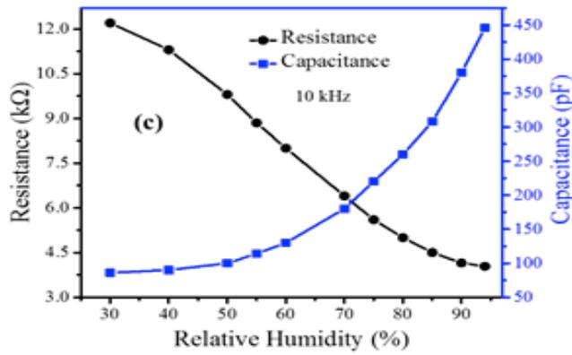
Figure 1: Resistance vs RH (black curves) and capacitance vs RH (blue curves) trends at (a) 0.1 kHz, (b) 1 kHz and (c) 10 kHz. The decrease in resistance and increase in capacitance manifests the humidity sensitivity of the device
