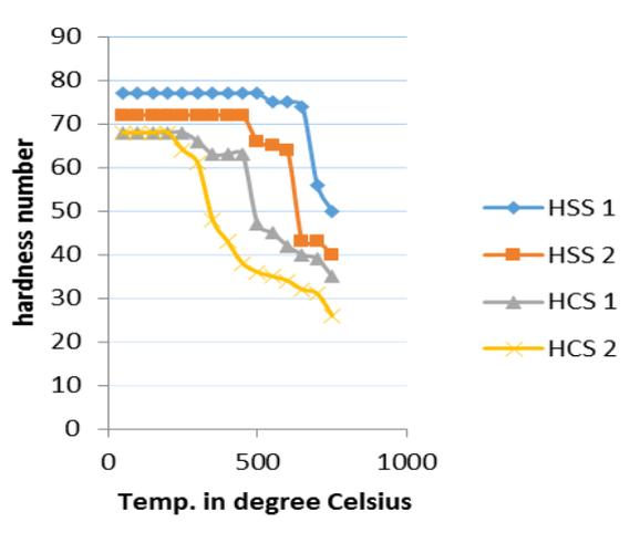
Fig. 4. Hardness Variation with Temperature
