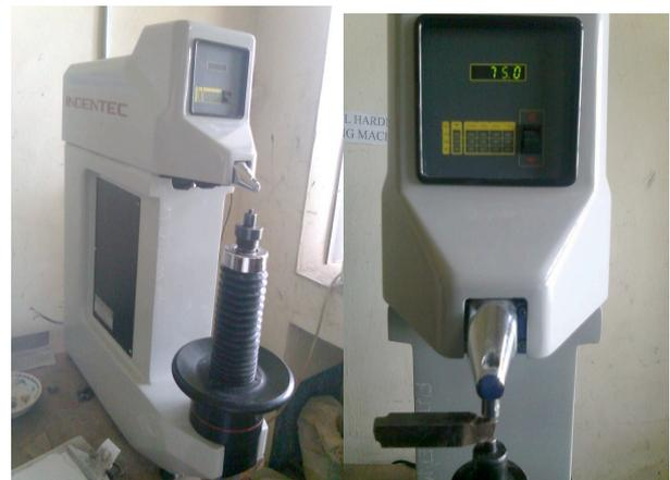
Fig. 2 Model -4150AK Digital Rockwell Hardness Testing Machine
