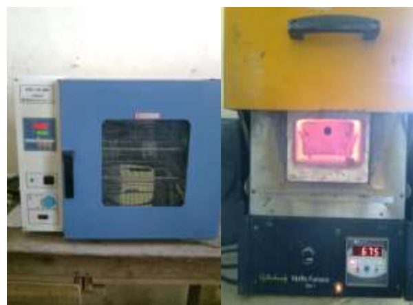
Fig. 3. Digital Electric furnace (Blast Air Oven of KX350A Model)
