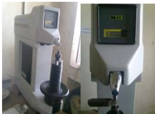
Fig. 2 Model -4150AK Digital Rockwell Hardness Testing Machine
