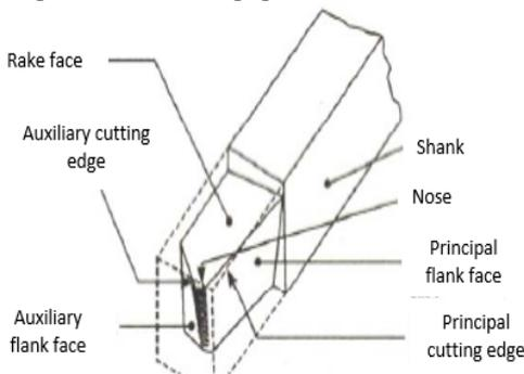
Fig. 1. Single point cutting tool geometry
