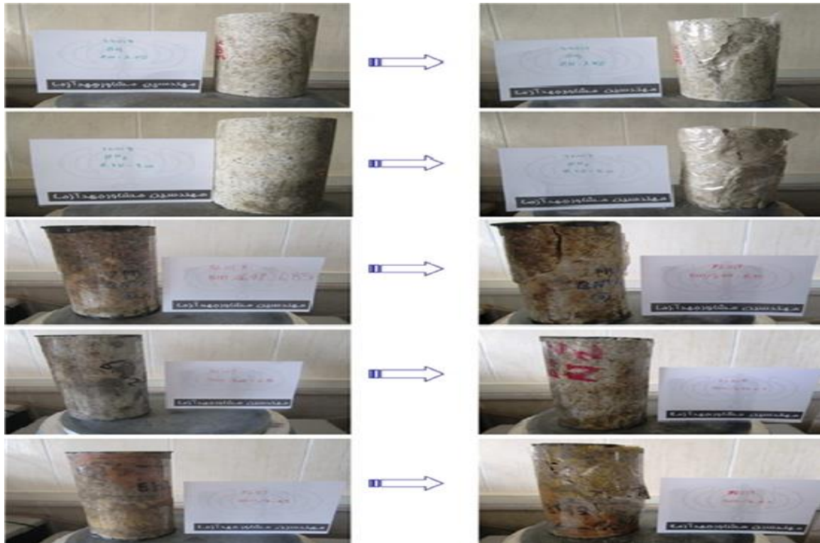
Fig 2. Samples condition in uniaxial compressive: Before the test on the left and after it on the right.
