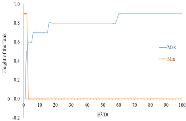
Fig. 6: Location of maximum and minimum hoop tension along the height of the tank wall v/s  $H^2/Dt$
