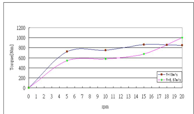
Fig.10 two torque curves for  $V=8.67\text{m/s}$  and  $V=10\text{m/s}$
