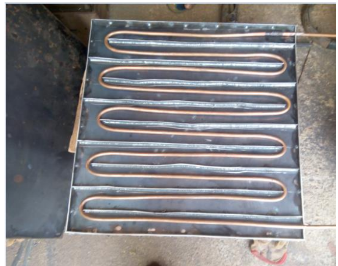
Fig no 6. Pipes and baffles
