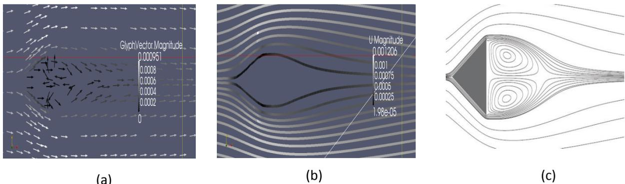
**Figure 5-** Simulation of flow around a triangular obstacle at Reynolds number 20
