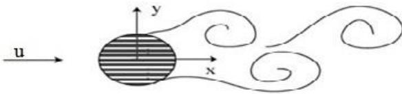
Figure 1- Vortex shedding when the fluid flows over an obstacle
