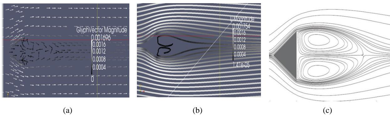
**Figure 7-** Simulation of flow around a triangular obstacle at Reynolds number 35
