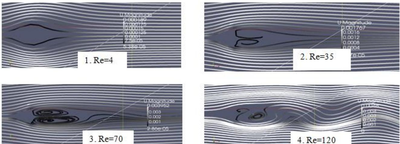
Figure 10- Flow patterns at Reynolds numbers of 4, 35, 70 and 120
