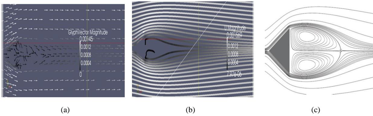
**Figure 6-** Simulation of flow around a triangular obstacle at Reynolds number 30
