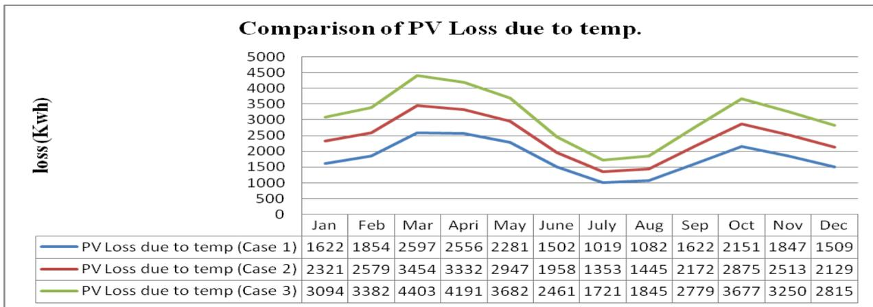
Figure 9. Comparison of PV loss due to temperature
