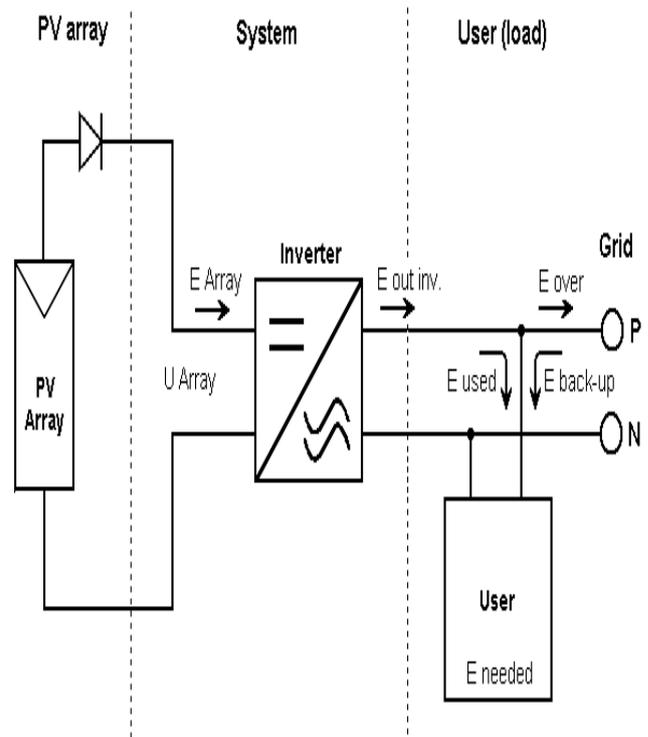
Figure 1. Block Diagram of Grid Connected PV system.
