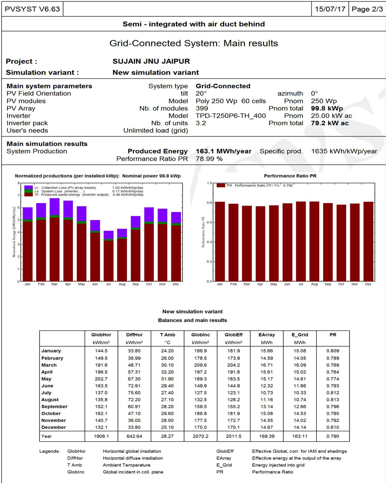
Figure 5. Performance ratio, nominal energy and monthly & yearly data of 100KW grid connected system(Case 2)
