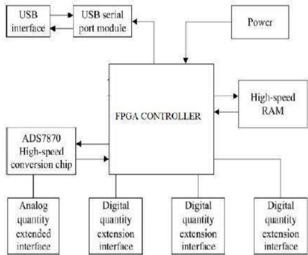
Fig2.2. FPGA HARDWARE BLOCK DIAGRAM
