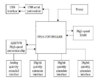
Fig2.2. FPGA HARDWARE BLOCK DIAGRAM
