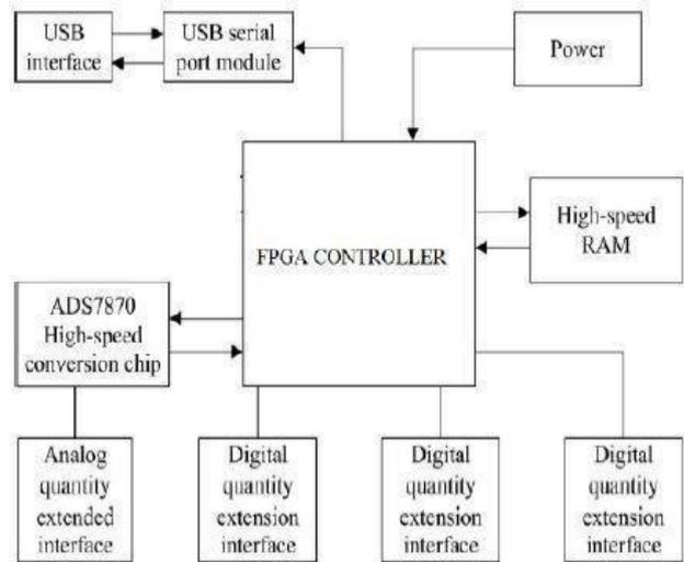
Fig2.2. FPGA HARDWARE BLOCK DIAGRAM
