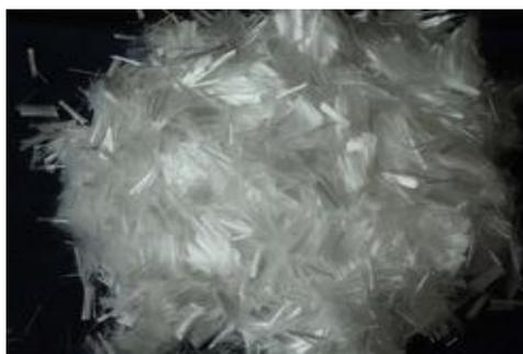
Fig 3. Polypropylene Fibres
