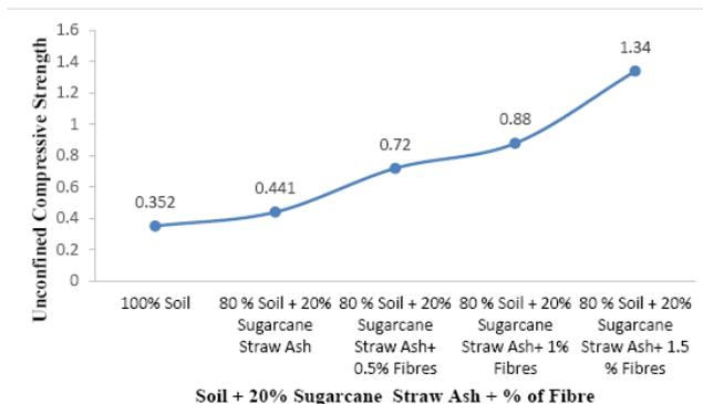
Fig. 7. Variation of Unconfined Compressive Strength for Soil + 20 % of Sugarcane Straw Ash + % of Polypropylene Fibres
