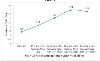
Fig.8. Variation of Soaked CBR Values for Soil + 20 % of Sugarcane Straw Ash + % of Polypropylene Fibres
