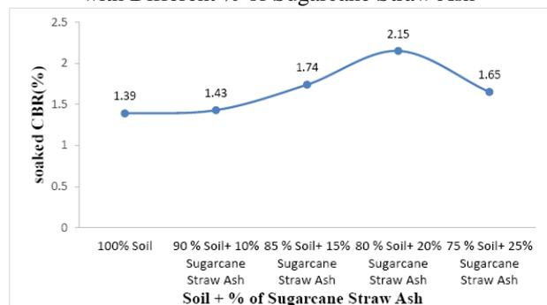
Fig. 6. Variation of Soaked CBR Values for Soil with Different % of Sugarcane Straw Ash
