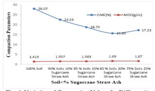
Fig. 4. Variation of Compaction Values for Different % Sugarcane Straw Ash Blended in Soil
