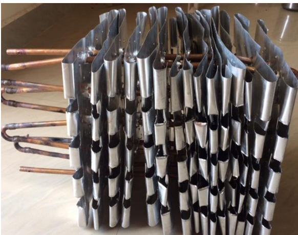
Fig.1.Multi-louvered plate fin dimpled, vortex generator
