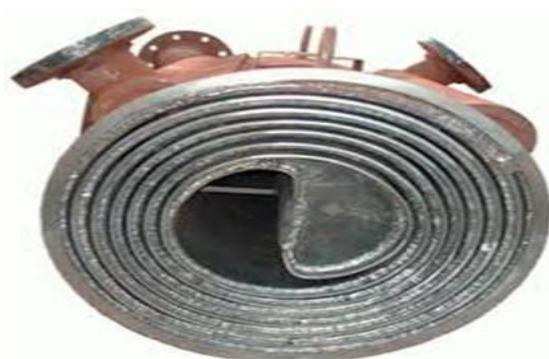
Fig 2. Cross sectional view of spiral plate.
