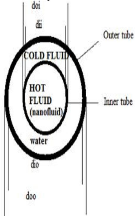
Fig 3. Double tube helical coiled tube
