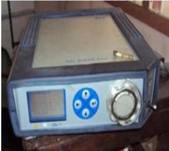
Figure 4: Photographic of AVL gas analyzer
