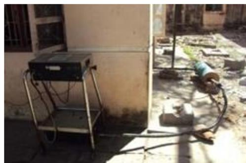
Figure 3: Photographic view of AVL smoke meter
