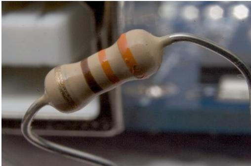
Fig. 3.4 Resistor
