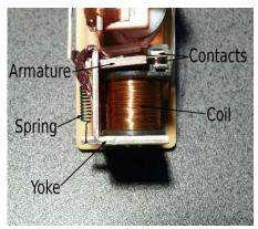
Fig. 3.2 Relay Switch
