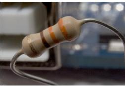
Fig. 3.4 Resistor
