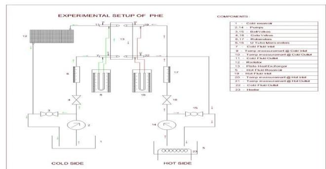
Figure 2. experimental layout of PHE
