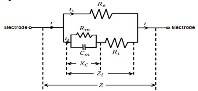
Fig. 1. The human body consists of resistors ( $R_e, R_m, R_i$ ) and Capacitor ( $C_m$ ) connected in parallel or in series. In the parallel model, two or more resistors and capacitors are connected in parallel, with the current passing through the extracellular space at low frequencies and through the intracellular space at high frequencies.
