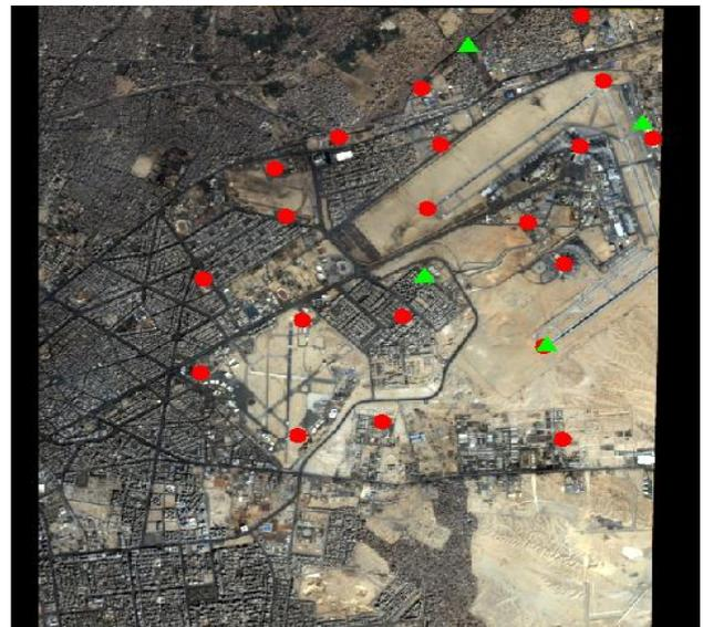
Fig. 3: Reference Image with distributed 20 point used as check points (red colors) & 4 GCPs with (green colors)
