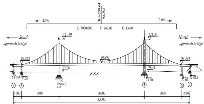
Figure1: elevation layout of bridge
