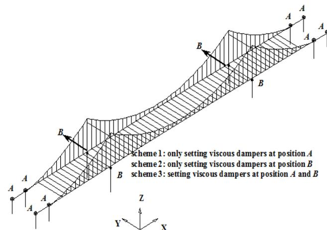
Fig. 2 Schematic diagram of viscous damper
