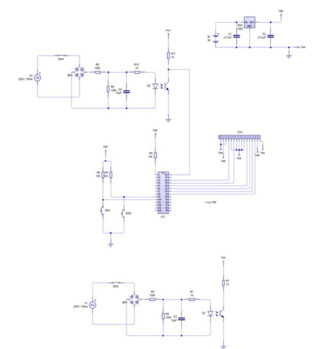
Figure 2: The Circuit Analysis of Power Failure Monitoring Data Logger System
