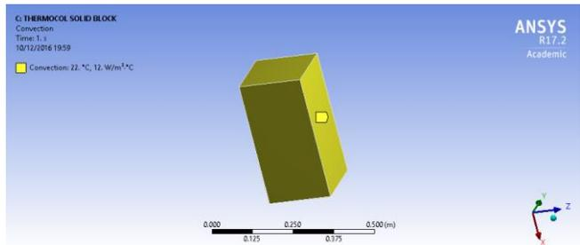
Fig .6. Convection of 12w/m<sup>2</sup>c added to five faces
