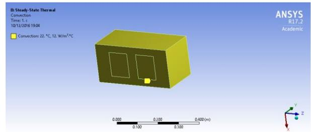
Fig .10. Convection of 12w/m<sup>2</sup>c added to five faces
