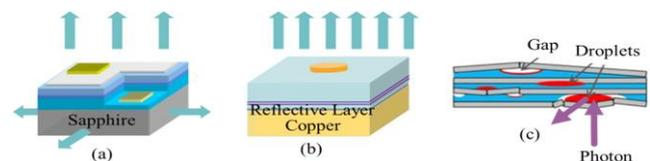
Fig. 1. Schematic structures of (a) a traditional lateral device, (b) typical substrate lifted vertical device and (c) SLS with Al droplets from post-LLO decomposition of low concentration Al<sub>x</sub>Ga<sub>1-x</sub>N.<sup>7)</sup>
