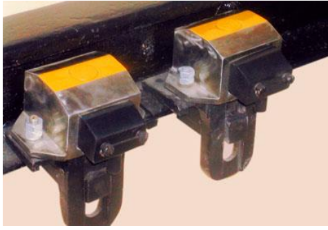
Fig. 2 Magnetic sensor mounted on the rails [6]
