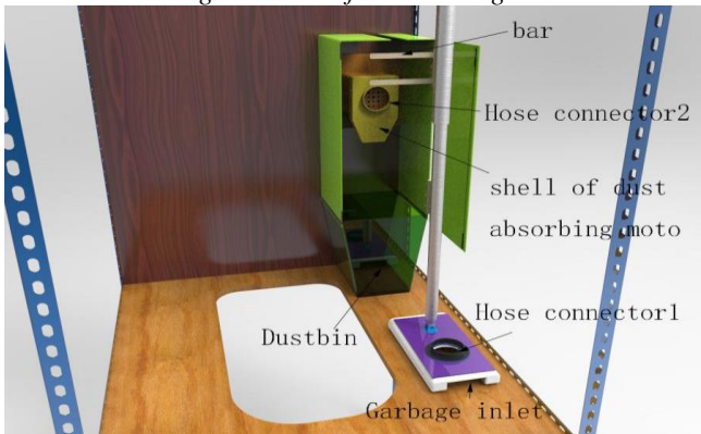
Fig. 10 Dust absorbing structure of the device.
