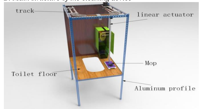
Figure 1 Model of cleaning device at working status.
