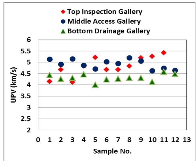
Fig 4 Results of UPV Test on the core samples from three galleries
