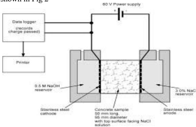
Fig. 2 RCPT Apparatus
