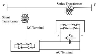
Figure 3. Schematic Diagram of UPFC Controller
