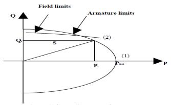
Figure 1. Capability curve of generator.
