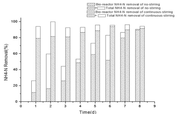
Fig.4 Ammonia nitrogen removal under non-stirring and continuous -stirring
