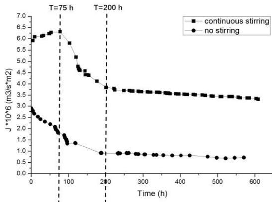
Fig.2 Variation of the membrane flux with time
