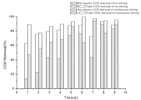
Fig.3 COD removal under non-stirring and continuous -stirring
