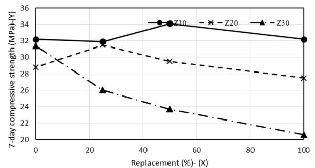
Fig 2. 7-day compressive strength of specimens
