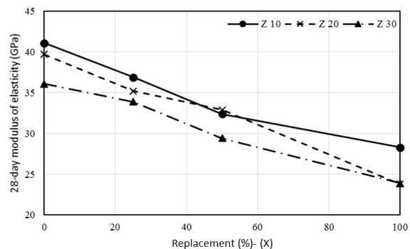
Fig 4. 28-day modulus of elasticity of specimens
