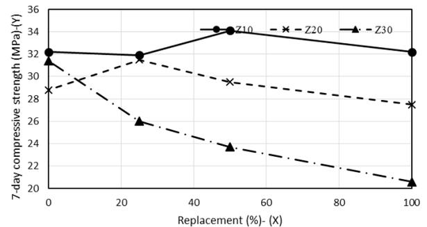
Fig 2. 7-day compressive strength of specimens
