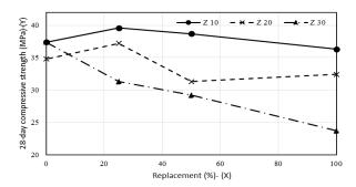
Fig 3. 28-day compressive strength of specimens
