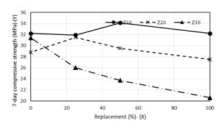
Fig 2. 7-day compressive strength of specimens
