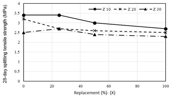
Fig 5. 28-day splitting tensile strength of specimens
