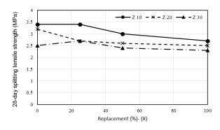
Fig 5. 28-day splitting tensile strength of specimens
