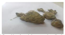
Fig 1. Presoaking of recycled aggregates in zeolite slurry
