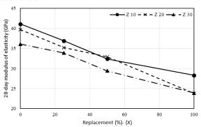
Fig 4. 28-day modulus of elasticity of specimens
