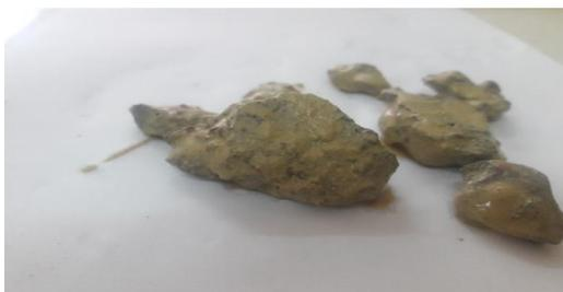
Fig 1. Presoaking of recycled aggregates in zeolite slurry
