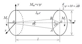
Fig 2. Torque elastic momentum and deformation during torquing of the main shaft.
