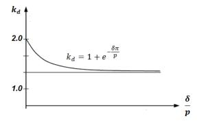
Fig 4. The dependence of the maximum value of the torsion elastic from the ratio  $\delta p$
