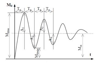
Fig 3. Replacement of elastic torsion moment depending on the time
