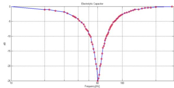
Fig. 4 Experimental measured frequency response of the designed notch filter
