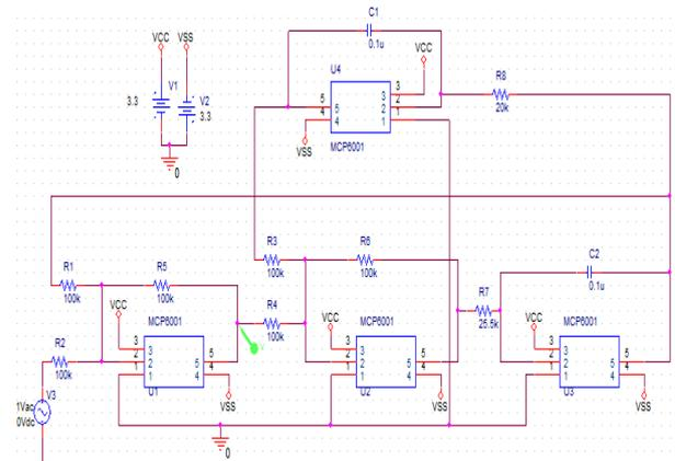
Fig. 3 Circuit diagram of the notch filter designed with MCP6400
