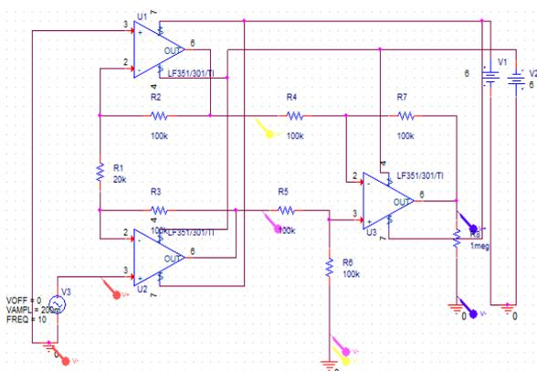
Fig. 2 Circuit diagram of the designed measurement amplifier
