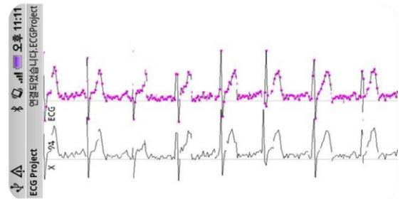
Fig. 7 Screen shot of Android Application showing real-time ECG graph
