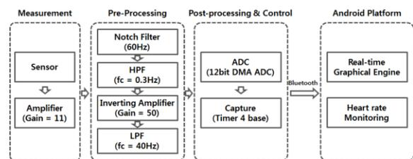
Fig. 1 Block diagram of the proposed ECG system
