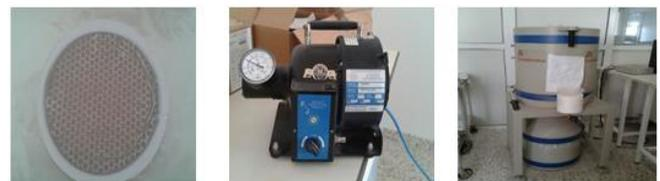
Fig 2: The equipment of experimental setup (a) filter (b) air pump and (c) HPGe detector
