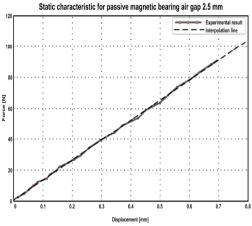
Fig 6: The static characteristic of passive magnetic bearing
