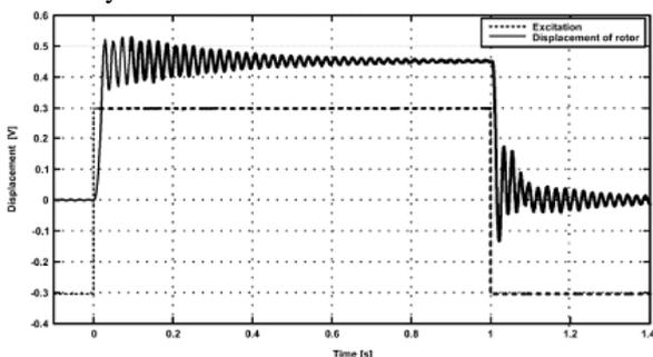
Fig 9: The step response of the PMB
