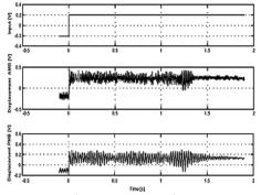
Fig 8: Step response of active (AMB) and passive (PMB) magnetic bearing to excitation by external signal at the axis Oy.
