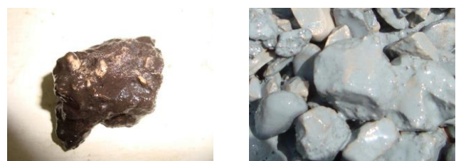
Fig 1. Presoaking of recycled aggregates in a) fly ash slurry b) silica fume slurry
