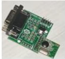
Fig.6 ZigBee Module
