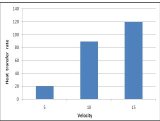
Figure 3: Heat dissipation and air velocity
