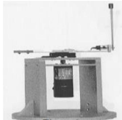
Fig1. Rotary inverted pendulum
