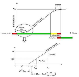
Figure 2: Concept of developed startup delay estimation model
