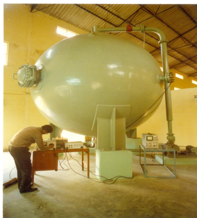
Fig.1. Large- 3.66-m diameter Spherical Vessel for explosion research studies
