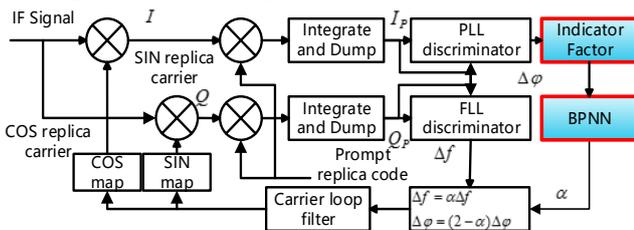
Fig. 2. Scheme of the advanced carrier tracking loop.
