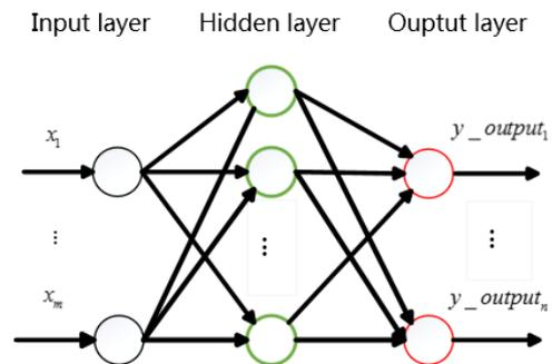
Fig. 3. A three-layer of back-propagation neural network
