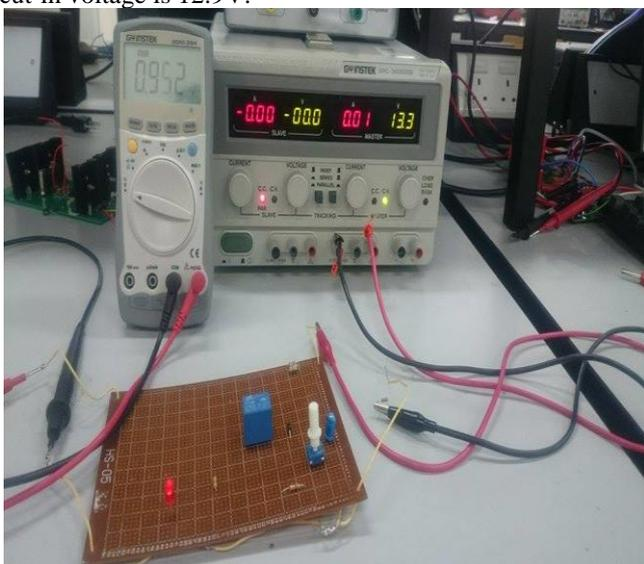
Fig. 6a: At 13.3V from the power supply, the relay cuts off the circuit.
