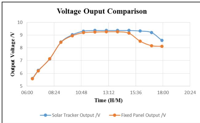
Fig. 11a: Output voltage comparison on day 1.
