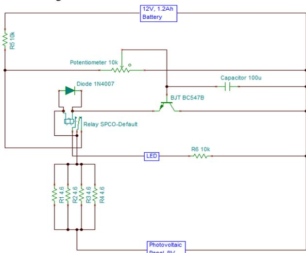
Fig. 5: Circuit schematic of the analogue charge controller.
