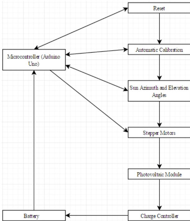
Fig. 1: Block schematic of the system operation.
