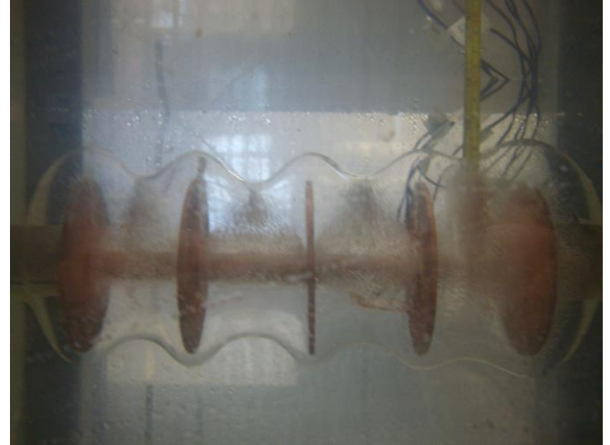
Figure 2 Photograph of the finned tube showing the solidified PCM and thermocouples for temperature measurements.
